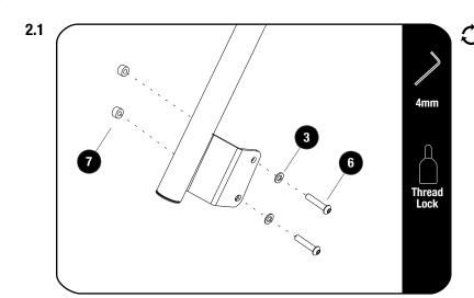
Align the holes in the Front Pillar Bracket mount plate with the holes on the vehicle. Loosely assemble the Pillar Bracket to the vehicle using M8 x 45 Button Head Bolts, M8 SS Spring Washers, M8 x 16 x 1.6SS Flat Washers and the spacers (Items 3, 6 & 7) as shown.
