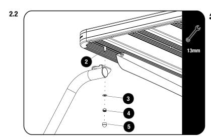
Fit your Roof Rack to the Front Support Arms using M8 x 20 Hex Bolts, M8 x 16 x 1.6SS Flat Washers and M8 Nyloc Nuts (Items 2, 3 & 4) as shown.
