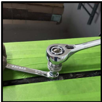
compress the plusnut by using a 1/2" wrench to hold the coupler & tighten with an 7/16" wrench
