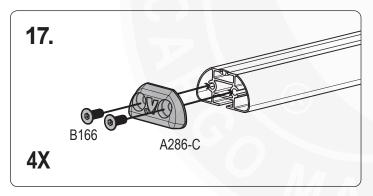
After adjusting the cross bar and uprights to align correctly and centered Tightly secure all hardware.
