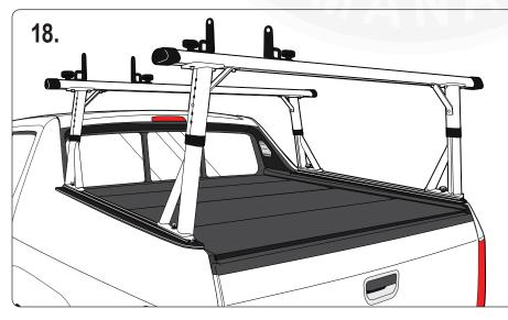
The truck bedrails taper towards the rear, loosen connections between cross bars and uprights. to allow for adjustments or removal of the rack system.
