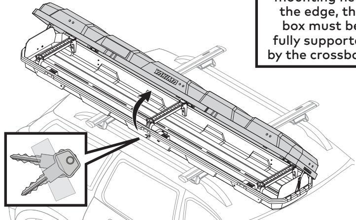
**Note:** If mounting near the edge, the box must be fully supported by the crossbars.
