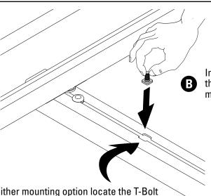
Insert the two T-Bolts through the entry point, and then proceed with steps 3 through 5 to secure the mounting bracket, and install you spare tire.
