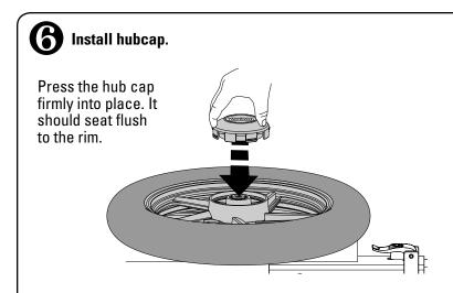
Note: To remove the hubcap use a flathead screwdriver to gently pry it from the rim.
